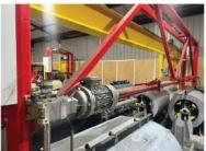
Fully automated slitting/cut to length line suitable for the sheet metal from coils, including an automated coil handling and coil warehousing system
